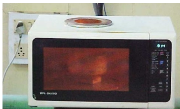
Figure 1. Modified domestic microwave oven used for synthesis of \text{SrLa}_y\text{Fe}_{12-x-y}\text{Cr}_x\text{O}_{19} .
